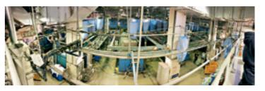
conveying system, offering washing capacity of over 64 tons per day. The system drastically reduces water consumption as water after rinsing and extraction will be reused for pre-wash. Moreover, its batch dryer is equipped with linen temperature sensing system which can optimise drying time in drying process and save energy.
